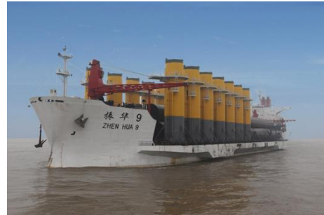
Figure 12: Shanghai Zhenhua Heavy Industry monopile transportation
